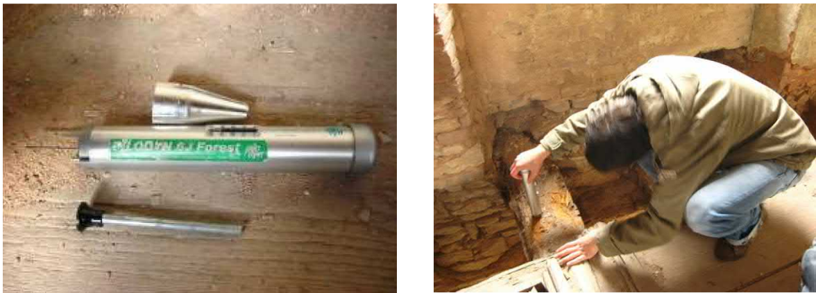
Figure 4. Pilodyn tool and its use for historic timber structures [22, p. 41].
